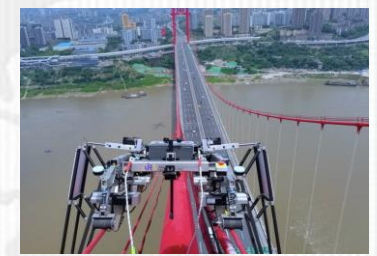
Bridge maintenance robot
