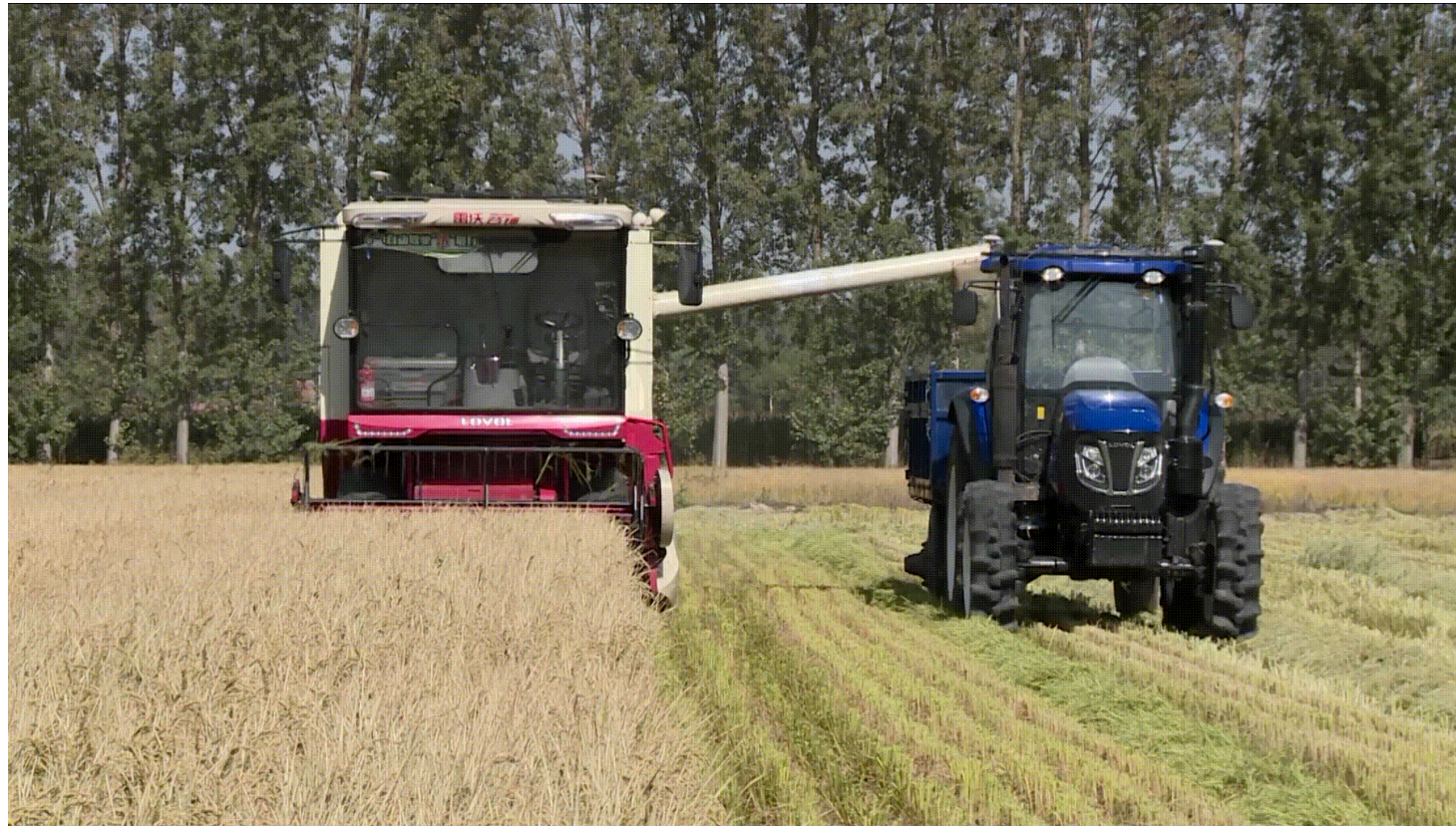
跟车卸粮模式 Unloading while Following the Vehicle
