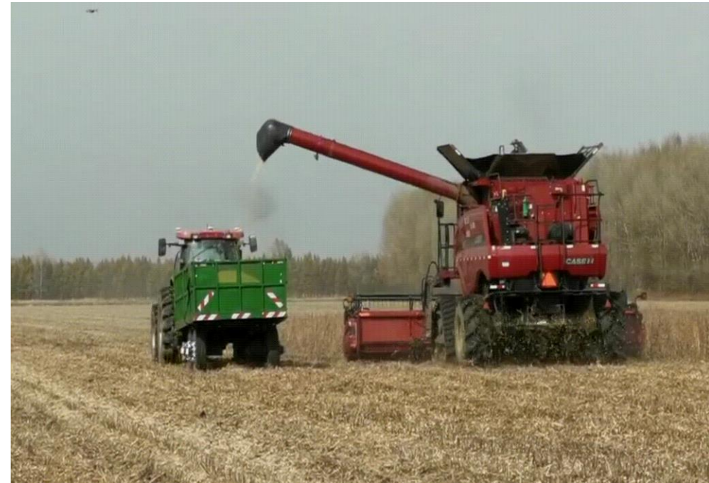
跟车卸粮模式 Unloading while Following the Vehicle
