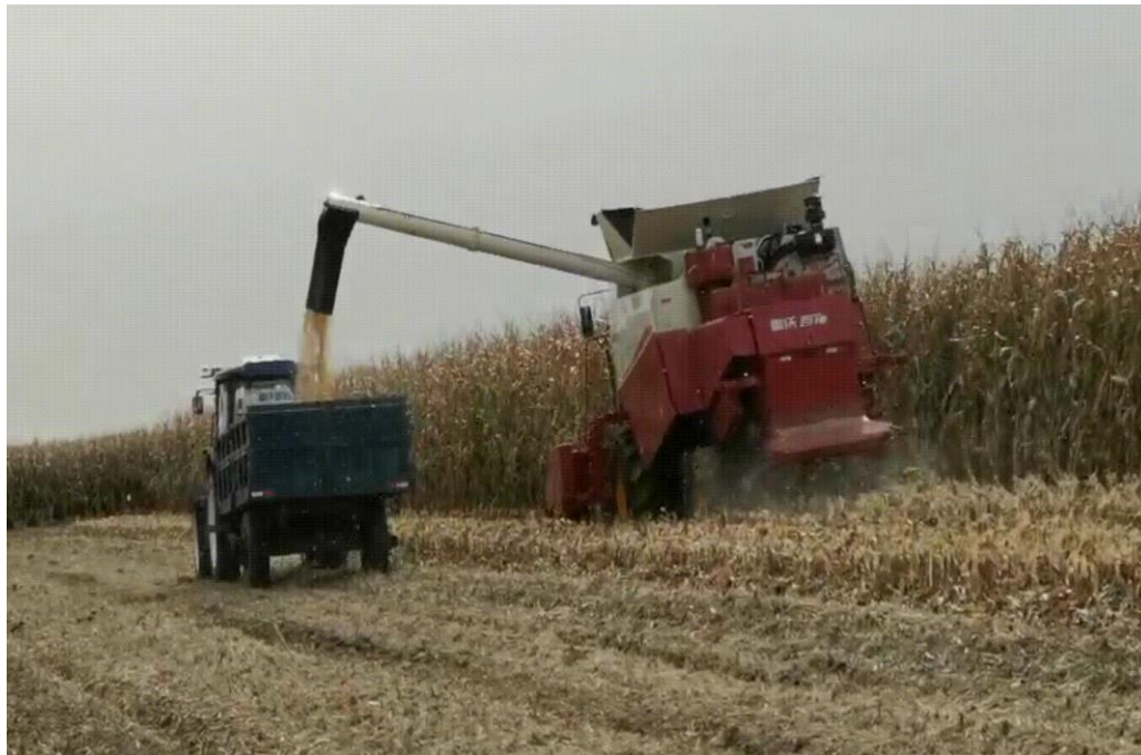
跟车卸粮模式 Unloading while Following the Vehicle
