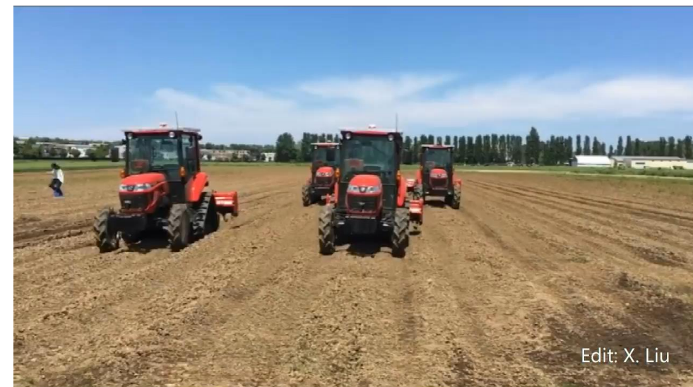
Robot farming system using multiple robot tractors
