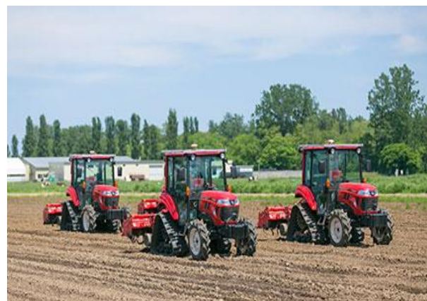
Robot farming system using multiple robot tractors
