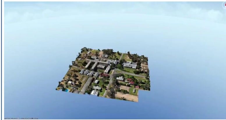
3D mesh scene constructed by oblique photos
