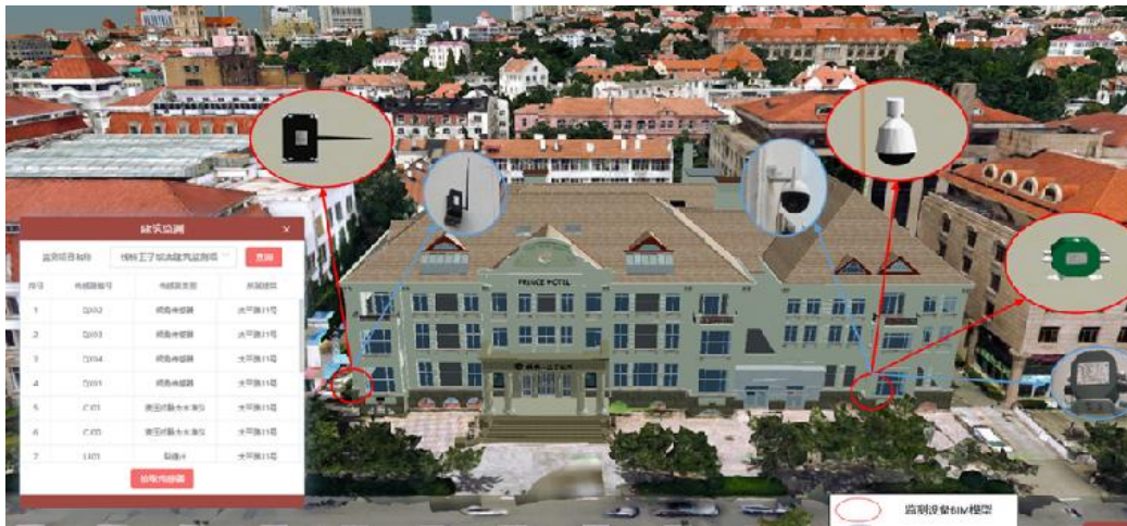
Fig 3-20 Integration of Monitoring Sensors with 3D Real Scene Geographic Scenes
