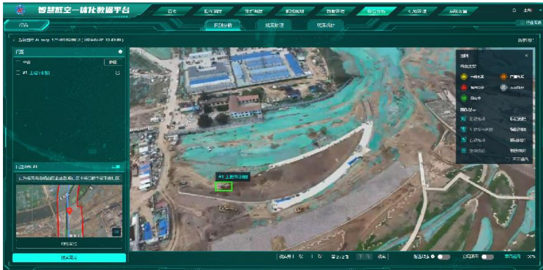
Fig 3-15 AI Automatic Recognition of Construction Vehicles from Video feeds
