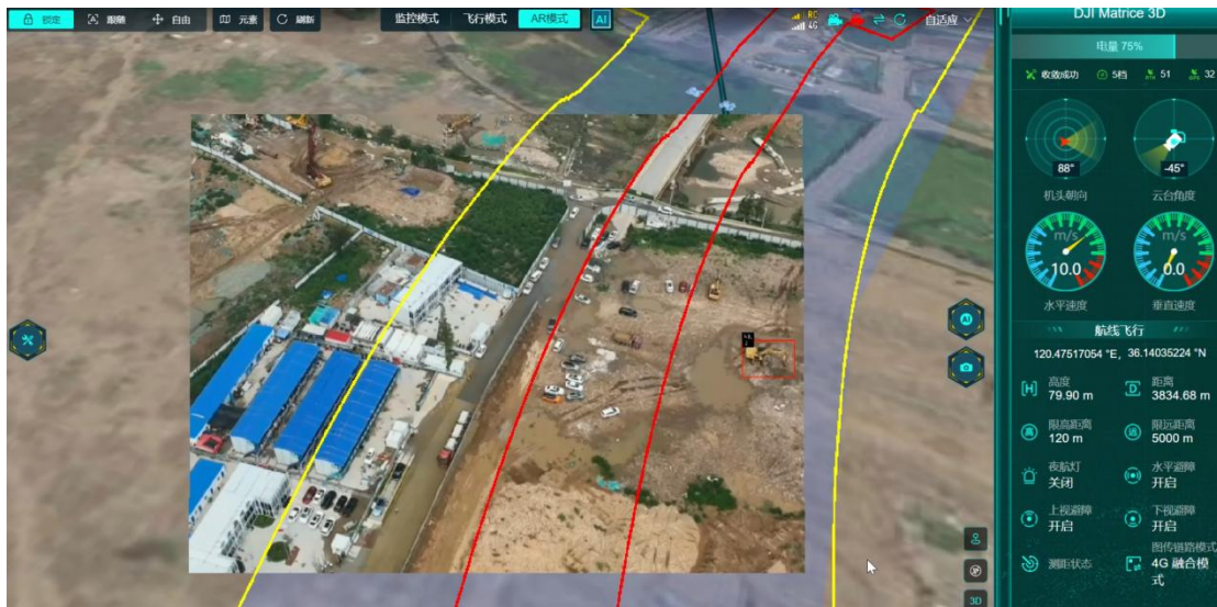
Fig 3-16 Drone Automated Inspection Route Setup
