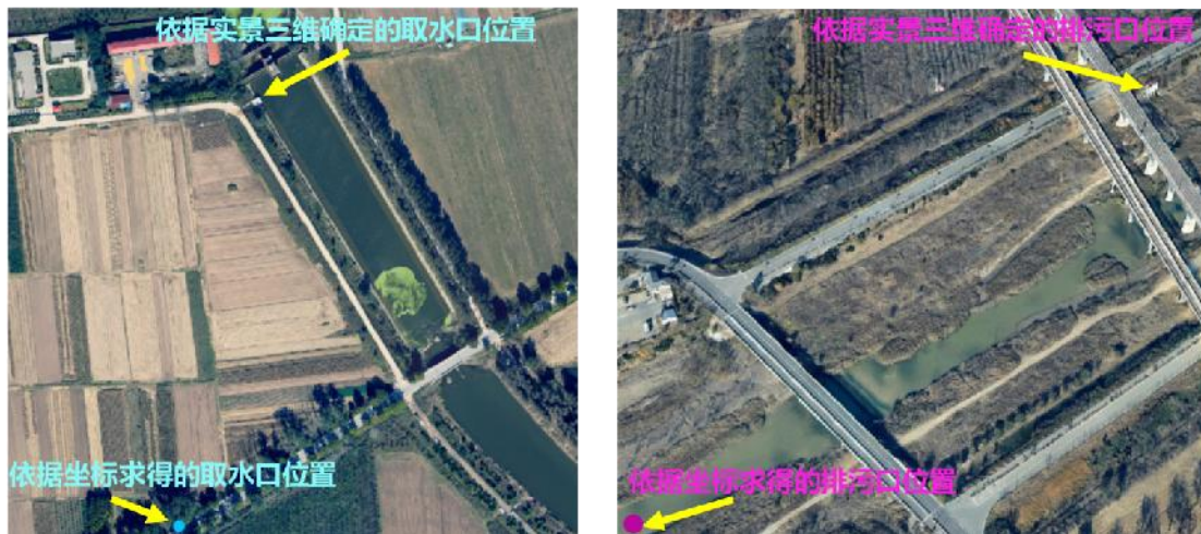
Figure 3-8 Accurate Positioning of Water Intake and Discharge Points Using 3D Real Scene
