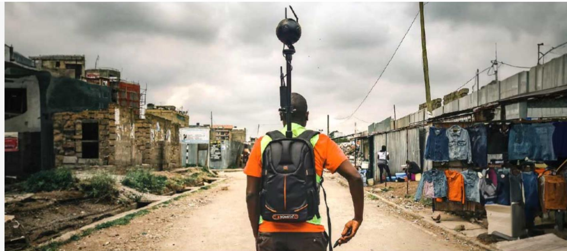
A worker walks through his settlement with a 360-degree terrestrial camera to capture Street View images. Photo: Spatial Collective
