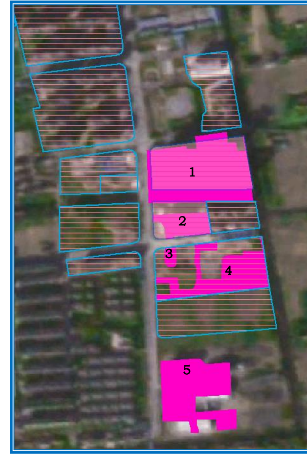
Fig. 6. The spots of newly-increased construction land overlay the spatial information of the approved construction land.
