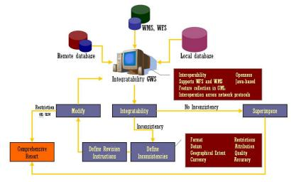
Figure 9: Components of integration GWS
