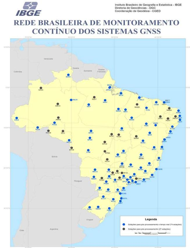
**Figure 3: Distribution of the current 101 RBMC stations. Blue dots (74) represent real-time and post-mission stations, whereas black dots (27) represent post-mission stations**
