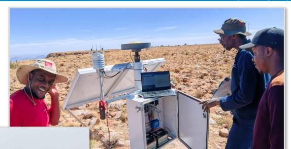
Self-contained Geodetic GNSS reference stations with full weather systems.
