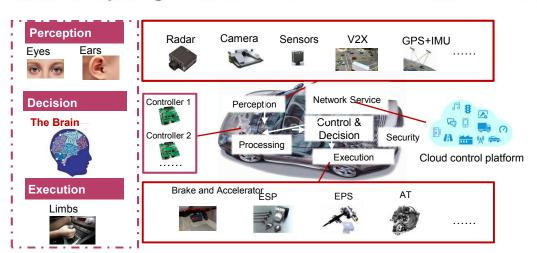
The computing platform (software& hardware platform) perceives real-time external environment through high-performance computing technology and highly trusted software, and optimize control and decision for the vehicle, it is the core of autonomous driving technology, and the dominating position in the development of ICV.
