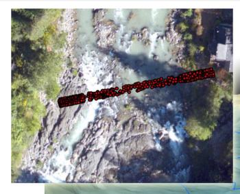
Ground Water Surface Bathymetry The top left image is the orthoimagery with a cross section of LiDAR returns in red. The middle image is a 3D representation of the gridded bathymetric model with classified LiDAR cross section. The bottom image is the LiDAR alone highlighting two pools in the river.
