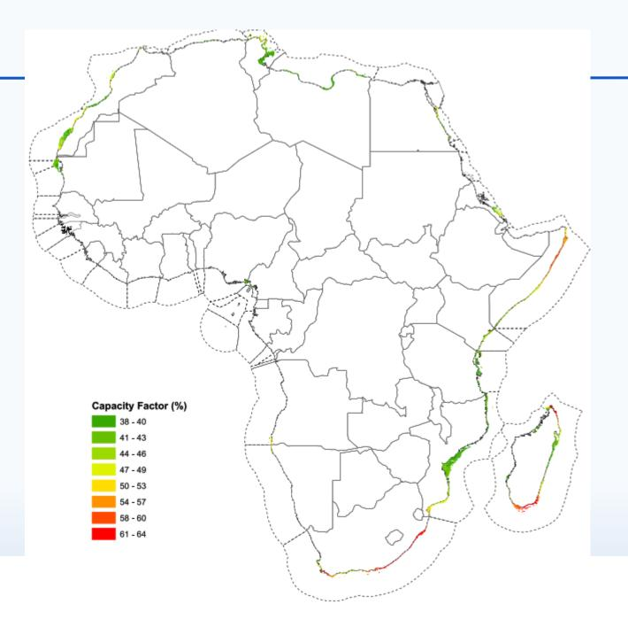
Capacity factor for waters shallow than 50m and up to 50 NM from the coast
