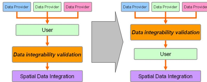
Figure 6: New approach for data integrability validation
