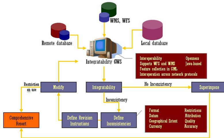
**Figure 9:** Components of integration GWS
