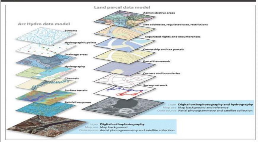
This is a schematic of the various types of layers that can be used in a GIS.
